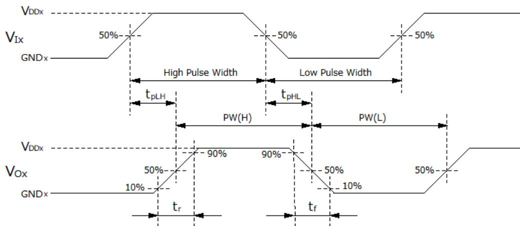
Figure12.4 Switching Waveforms
