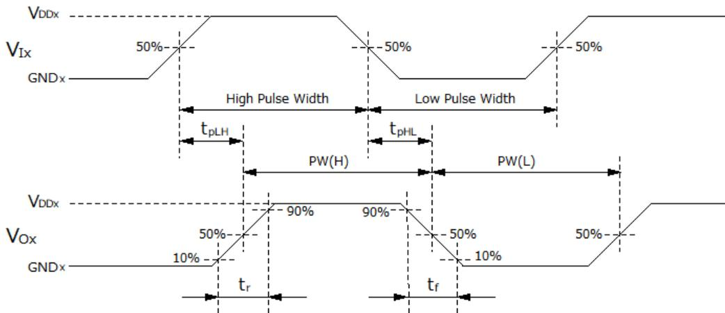
**Figure12.4 Switching Waveforms**
