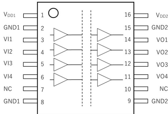
**Figure 6.1 Pin Assignments (top view)**
