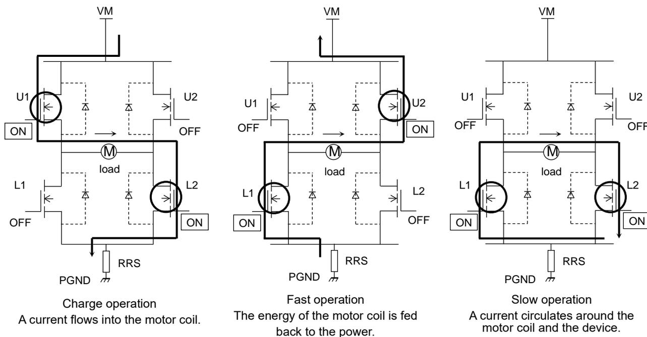
**Figure 9.1 Operation Mode of Output Transistor (Positive Current)**
