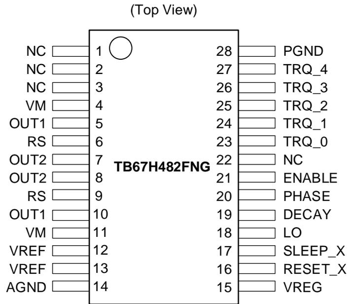
**Figure 5 Pin Assignments**
