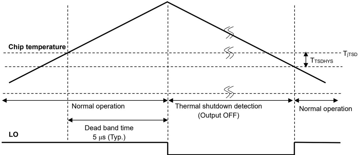
**Figure 11.1 Thermal Shutdown Detection Timing Chart 1**
