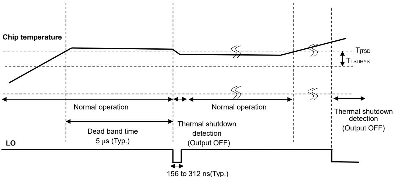
**Figure 11.2 Thermal Shutdown Detection Timing Chart 2**
