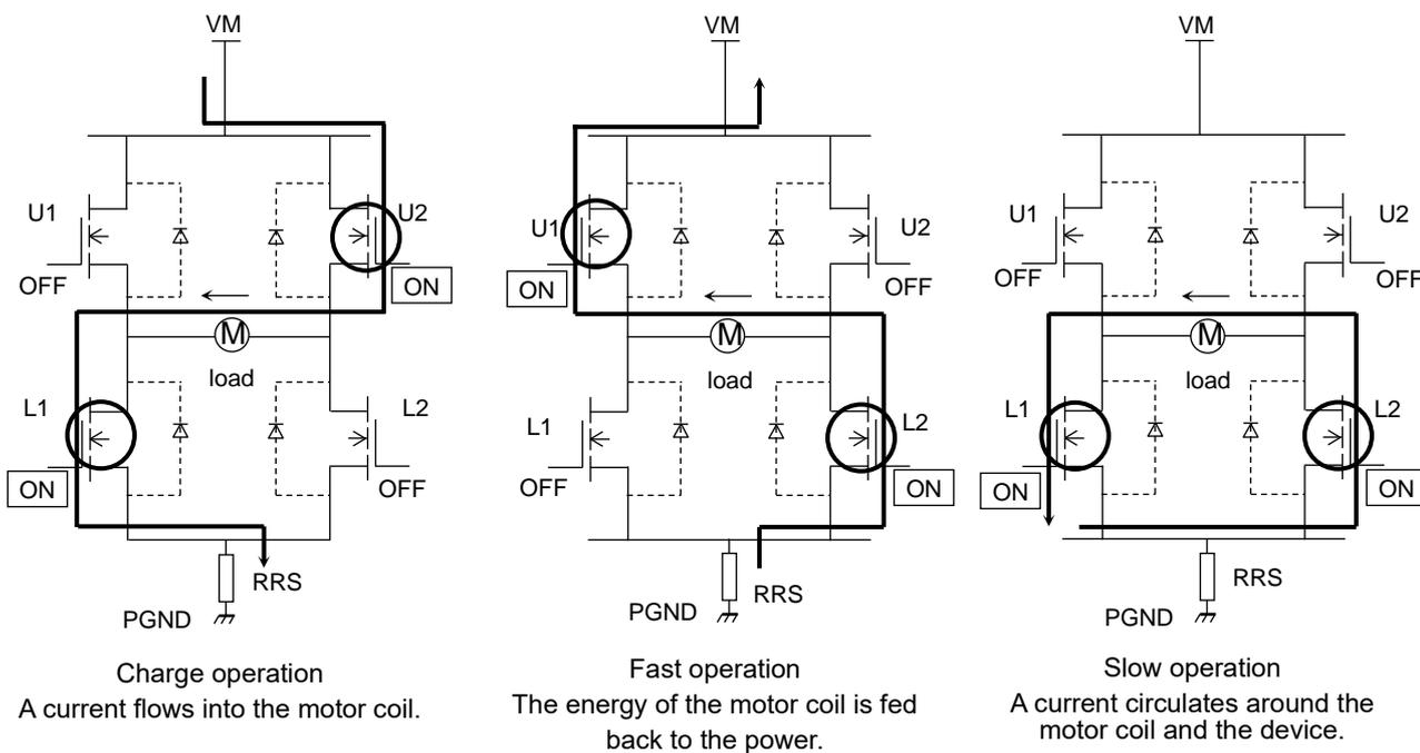
**Figure 9.2 Operation Mode of Output Transistor (Negative Current)**
