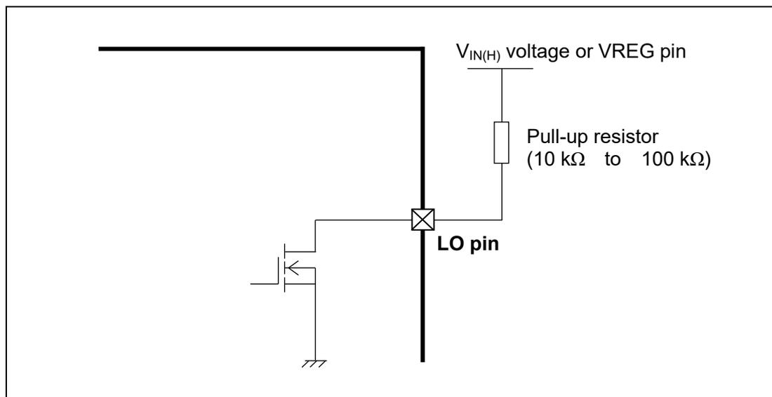
**Figure 8.2 LO pin equivalent circuit diagram**
