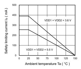
Thermal derating curve for safety limiting current - Ta
