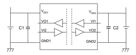
Figure 8.1 Pin Assignments (top view)
