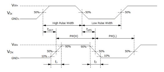
Figure 12.4 Switching Waveforms
