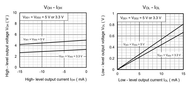
Figure 12.2 Output Voltage - Output Current
