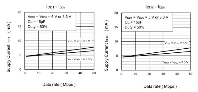
Figure12.1 Supply Current - Data rate
