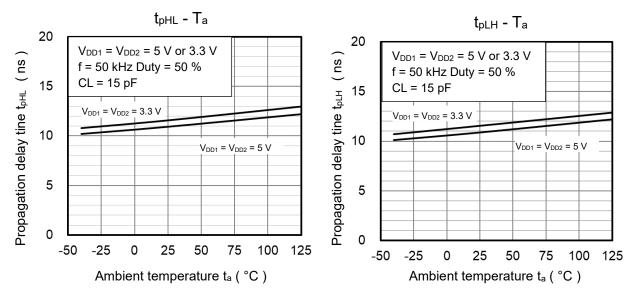
Figure 12.3 Propagation Delay Time vs Ambient Temperature
