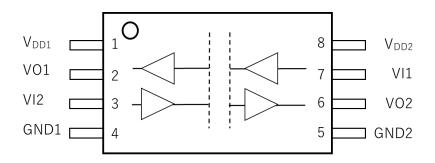
Figure 6.1 Pin Assignments (top view)
