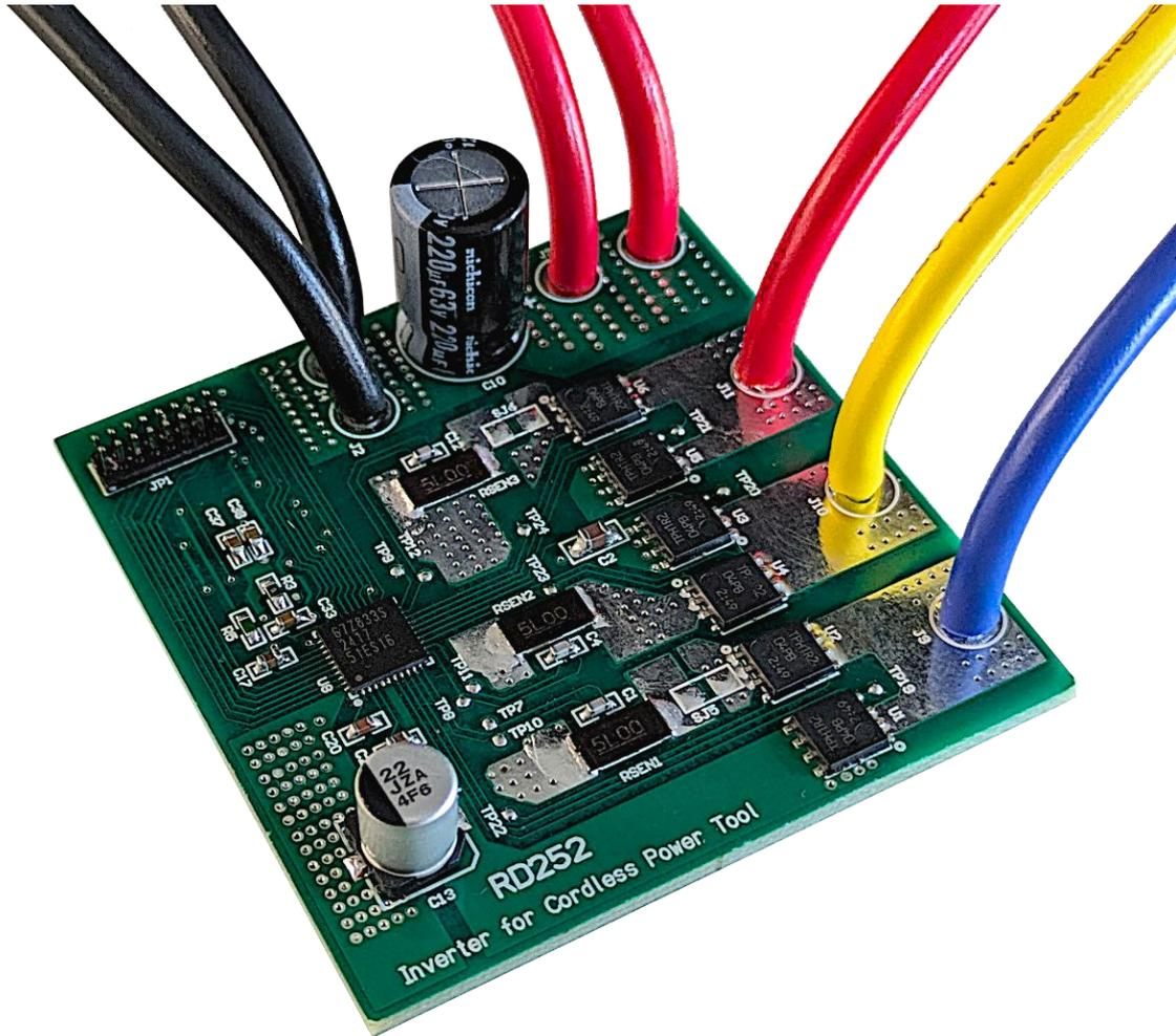
Fig. 2.4 Board of This Design (Side View)
