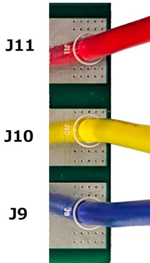
**Fig. 4.1 Motor Connection**
