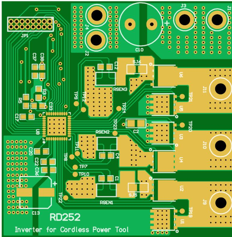
**Fig. 2.5 Layout of Main Components (Top View)**
