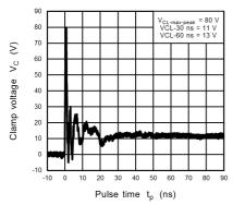
Fig. 11.7.5 ISO10605 Clamp Waveform +8 kV
