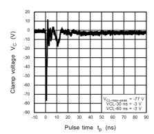
Fig. 11.20.6 ISO10605 Clamp Waveform -8 kV
