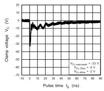
Fig. 11.21.4 IEC61000-4-2 Clamp Waveform -8 kV
