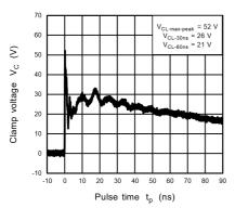
Fig. 11.15.3 IEC61000-4-2 Clamp Waveform +8 kV
