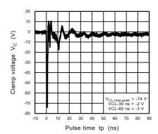
Fig. 11.6.6 ISO10605 Clamp Waveform -8 kV
