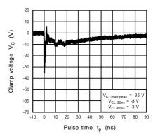
Fig. 11.5.4 IEC61000-4-2 Clamp Waveform -8 kV
