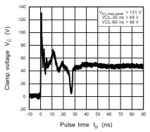
Fig. 11.21.5 ISO10605 Clamp Waveform +8 kV
