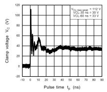
Fig. 11.18.5 ISO10605 Clamp Waveform +8 kV
