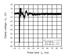
Fig. 11.14.6 ISO10605 Clamp Waveform -8 kV
