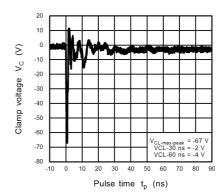
Fig. 11.15.6 ISO10605 Clamp Waveform -8 kV
