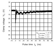
Fig. 11.17.4 IEC61000-4-2 Clamp Waveform -8 kV
