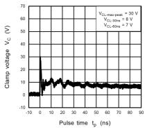
Fig. 11.2.3 IEC61000-4-2 Clamp Waveform +8 kV
