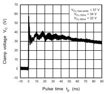
Fig. 11.17.3 IEC61000-4-2 Clamp Waveform +8 kV
