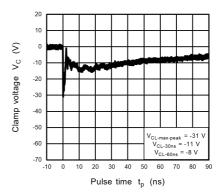
Fig. 11.7.4 IEC61000-4-2 Clamp Waveform -8 kV
