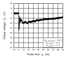
Fig. 11.11.4 IEC61000-4-2 Clamp Waveform -8 kV
