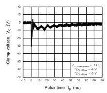
Fig. 11.13.4 IEC61000-4-2 Clamp Waveform -8 kV
