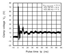
Fig. 11.6.5 ISO10605 Clamp Waveform +8 kV
