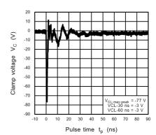
Fig. 11.18.6 ISO10605 Clamp Waveform -8 kV
