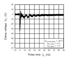
Fig. 11.16.4 IEC61000-4-2 Clamp Waveform -8 kV
