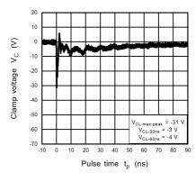
Fig. 11.4.4 IEC61000-4-2 Clamp Waveform -8 kV
