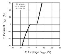
Fig. 11.5.1 I<sub>TLP</sub> - V<sub>TLP</sub>
