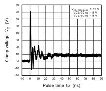
Fig. 11.4.5 ISO10605 Clamp Waveform +8 kV
