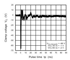
Fig. 11.3.6 ISO10605 Clamp Waveform -8 kV
