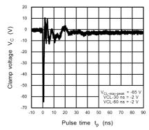
Fig. 11.8.6 ISO10605 Clamp Waveform -8 kV
