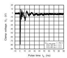
Fig. 11.21.6 ISO10605 Clamp Waveform -8 kV
