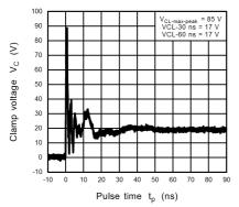
Fig. 11.13.5 ISO10605 Clamp Waveform +8 kV
