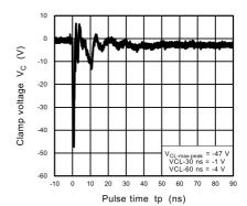
Fig. 11.5.6 ISO10605 Clamp Waveform -8 kV
