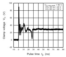
Fig. 11.17.5 ISO10605 Clamp Waveform +8 kV
