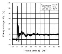
Fig. 11.5.5 ISO10605 Clamp Waveform +8 kV
