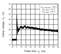
Fig. 11.12.3 IEC61000-4-2 Clamp Waveform +8 kV
