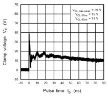
Fig. 11.6.3 IEC61000-4-2 Clamp Waveform +8 kV
