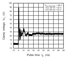
Fig. 11.16.5 ISO10605 Clamp Waveform +8 kV
