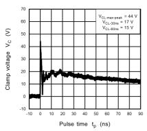
Fig. 11.8.3 IEC61000-4-2 Clamp Waveform +8 kV
