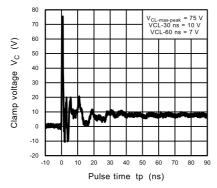
Fig. 11.3.5 ISO10605 Clamp Waveform +8 kV
