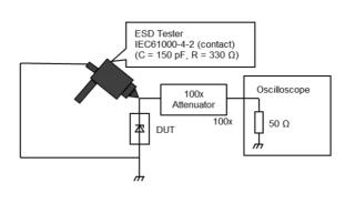
Fig. 11.22.2 Clamp waveform measurement circuit(according to IEC61000-4-2)
