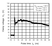
Fig. 11.18.3 IEC61000-4-2 Clamp Waveform +8 kV
