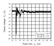
Fig. 11.7.6 ISO10605 Clamp Waveform -8 kV
