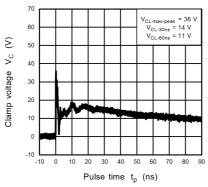
Fig. 11.5.3 IEC61000-4-2 Clamp Waveform +8 kV
