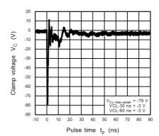
Fig. 11.19.6 ISO10605 Clamp Waveform -8 kV
