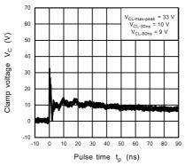
Fig. 11.3.3 IEC61000-4-2 Clamp Waveform +8 kV
