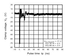
Fig. 11.4.6 ISO10605 Clamp Waveform -8 kV
