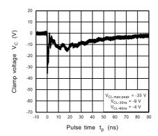
Fig. 11.10.4 IEC61000-4-2 Clamp Waveform -8 kV
