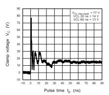
Fig. 11.9.5 ISO10605 Clamp Waveform +8 kV
