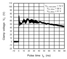
Fig. 11.20.3 IEC61000-4-2 Clamp Waveform +8 kV
