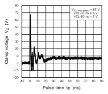
Fig. 11.2.5 ISO10605 Clamp Waveform +8 kV
