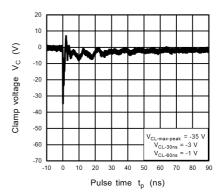
Fig. 11.2.4 IEC61000-4-2 Clamp Waveform -8 kV
