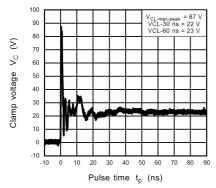
Fig. 11.15.5 ISO10605 Clamp Waveform +8 kV
