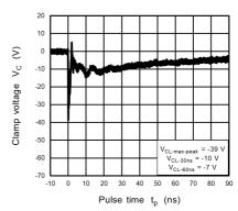
Fig. 11.8.4 IEC61000-4-2 Clamp Waveform -8 kV
