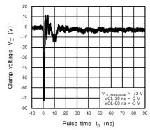
Fig. 11.17.6 ISO10605 Clamp Waveform -8 kV
