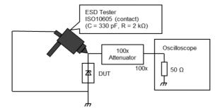
Fig. 11.22.3 Clamp waveform measurement circuit(according to ISO10605)
