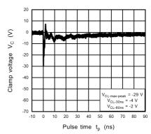
Fig. 11.3.4 IEC61000-4-2 Clamp Waveform -8 kV
