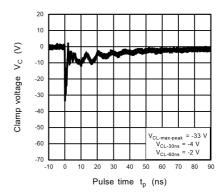
Fig. 11.18.4 IEC61000-4-2 Clamp Waveform -8 kV
