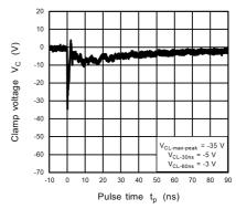
Fig. 11.15.4 IEC61000-4-2 Clamp Waveform -8 kV
