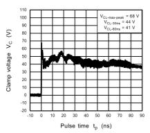
Fig. 11.19.3 IEC61000-4-2 Clamp Waveform +8 kV
