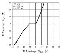
Fig. 11.9.1 I<sub>TLP</sub> - V<sub>TLP</sub>
