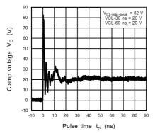
Fig. 11.14.5 ISO10605 Clamp Waveform +8 kV
