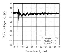
Fig. 11.12.4 IEC61000-4-2 Clamp Waveform -8 kV
