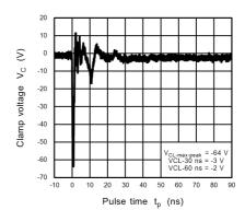
Fig. 11.16.6 ISO10605 Clamp Waveform -8 kV
