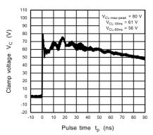
Fig. 11.21.3 IEC61000-4-2 Clamp Waveform +8 kV
