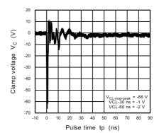
Fig. 11.2.6 ISO10605 Clamp Waveform -8 kV
