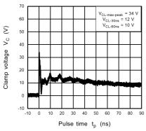
Fig. 11.4.3 IEC61000-4-2 Clamp Waveform +8 kV
