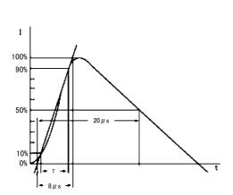
Fig. 11.22.1 V<sub>C</sub>-I<sub>PP</sub> Peak Pulse Current (according to IEC61000-4-5 8/20 μs pulse)
