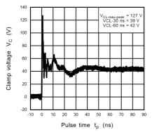
Fig. 11.20.5 ISO10605 Clamp Waveform +8 kV
