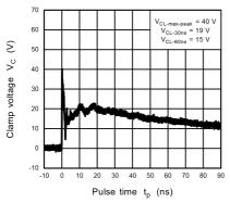
Fig. 11.7.3 IEC61000-4-2 Clamp Waveform +8 kV
