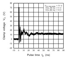
Fig. 11.8.5 ISO10605 Clamp Waveform +8 kV
