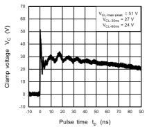
Fig. 11.14.3 IEC61000-4-2 Clamp Waveform +8 kV
