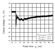
Fig. 11.9.4 IEC61000-4-2 Clamp Waveform -8 kV
