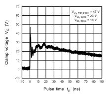
Fig. 11.10.3 IEC61000-4-2 Clamp Waveform +8 kV
