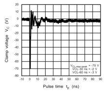
Fig. 11.13.6 ISO10605 Clamp Waveform -8 kV
