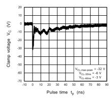
Fig. 11.19.4 IEC61000-4-2 Clamp Waveform -8 kV
