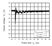
Fig. 11.14.4 IEC61000-4-2 Clamp Waveform -8 kV
