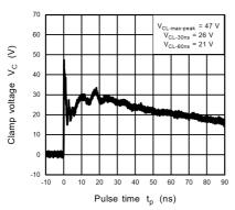
Fig. 11.11.3 IEC61000-4-2 Clamp Waveform +8 kV
