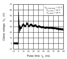
Fig. 11.16.3 IEC61000-4-2 Clamp Waveform +8 kV
