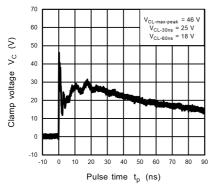
Fig. 11.9.3 IEC61000-4-2 Clamp Waveform +8 kV
