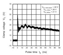
Fig. 11.13.3 IEC61000-4-2 Clamp Waveform +8 kV
