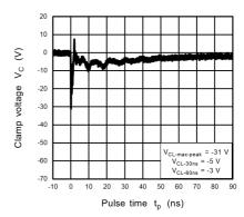
Fig. 11.6.4 IEC61000-4-2 Clamp Waveform -8 kV
