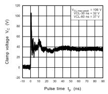
Fig. 11.19.5 ISO10605 Clamp Waveform +8 kV
