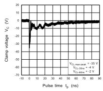
Fig. 11.20.4 IEC61000-4-2 Clamp Waveform -8 kV
