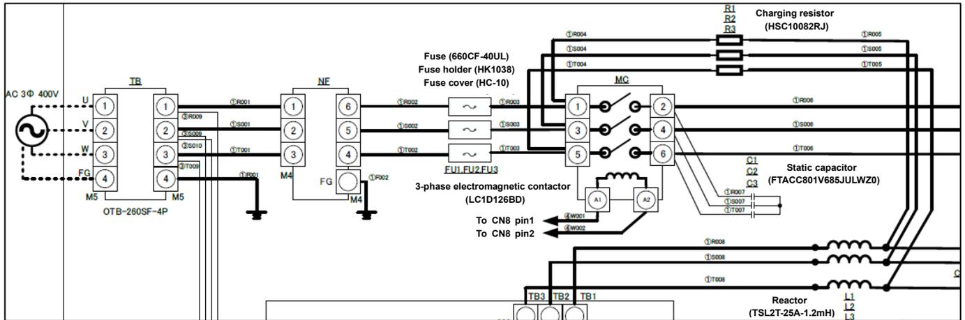
**Fig. 3.1 AC Line Circuit**
