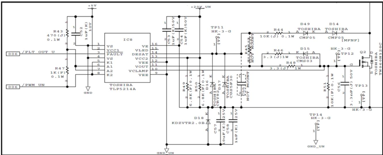
**Fig. 3.2 Gate Drive Circuit (U-Phase Lower Arm)**
