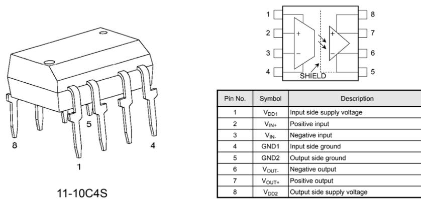
**Fig. 2.3 Appearance and Pin Configuration Diagram of TLP7920**
