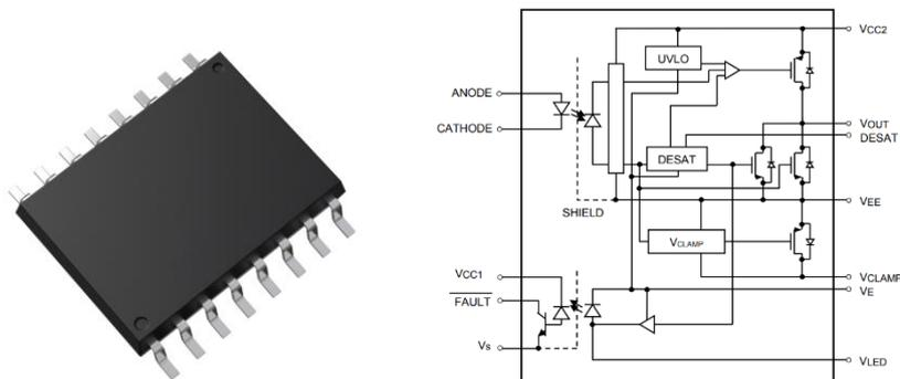
**Fig. 2.2 Appearance and Block Diagram of TLP5214A**
