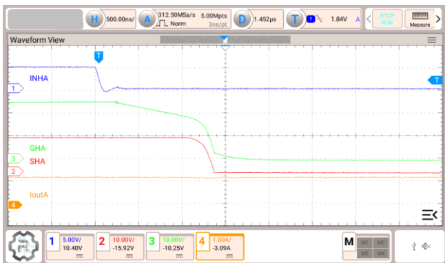
Figure 3.17 Isink = 60 mA, H-side, Positive current
