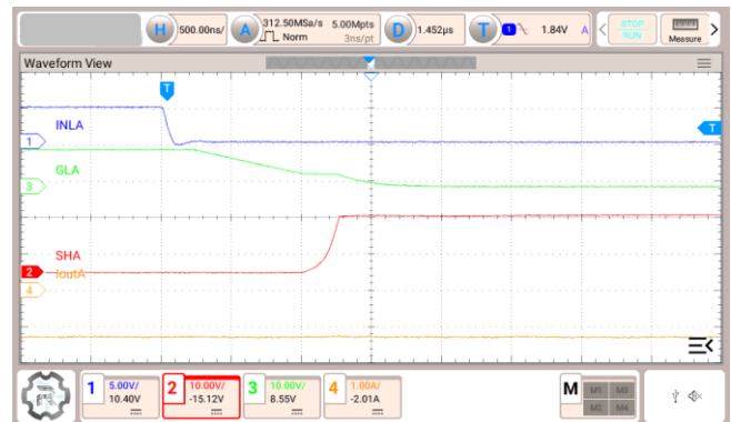
Figure 3.24 Isink = 60 mA, L-side, Negative current
