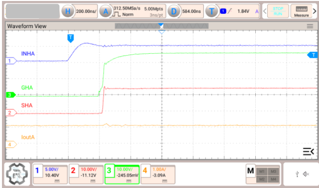
Figure 3.1 I source = 1 A, H-side, Positive current
