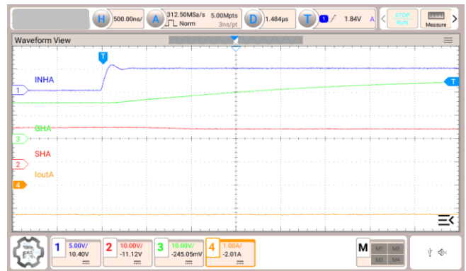
Figure 3.6 I source = 30 mA, H-side, Negative current
