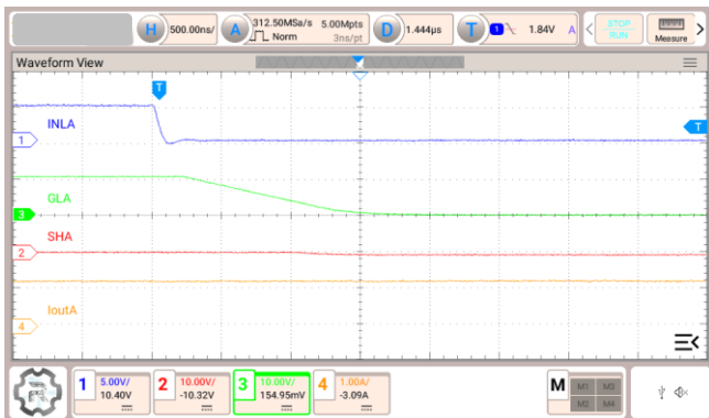
Figure 3.23 Isink = 60 mA, L-side, Positive current
