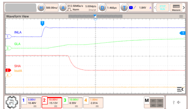
Figure 3.12 Isource = 30 mA, L-side, Negative current
