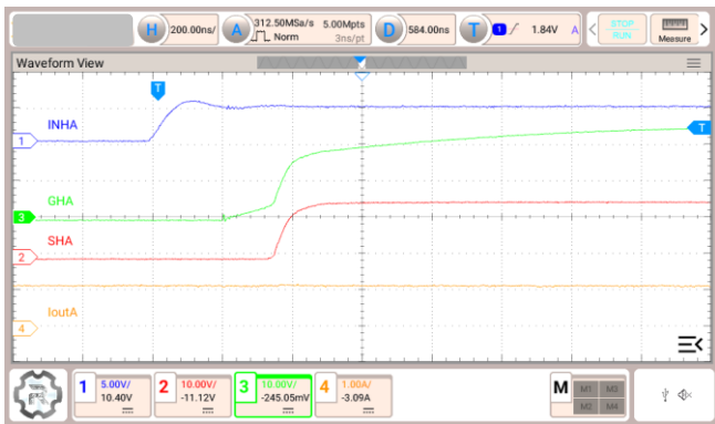
Figure 3.3 I source = 120 mA, H-side, Positive current
