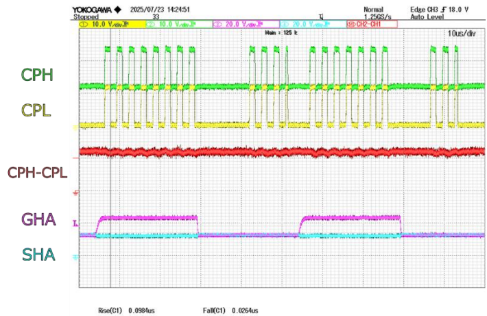
Figure 6.2 Charge pump waveform example
