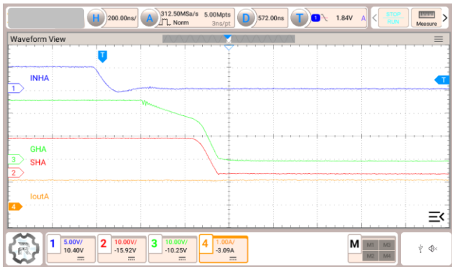
Figure 3.15 Isink = 240 mA, H-side, Positive current
