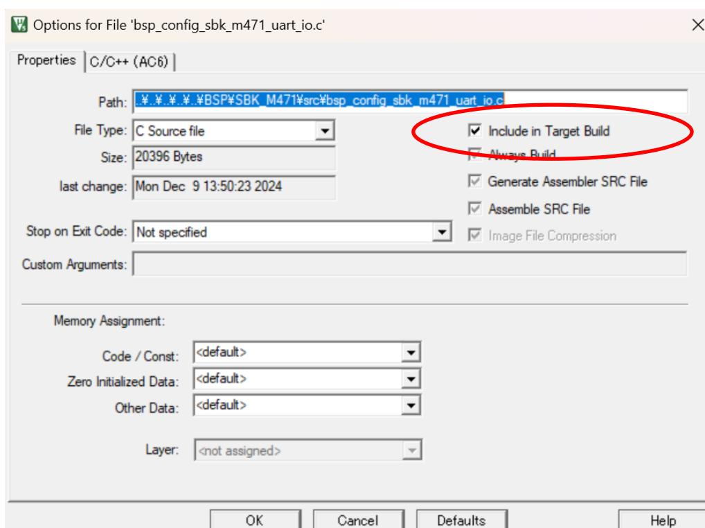
Right-click the file you want to configure, open Options for File 'xxxx.c' and change "Include in Target Build". If you want to use the file, check "Include in Target Build", otherwise uncheck "Include in Target Build".
