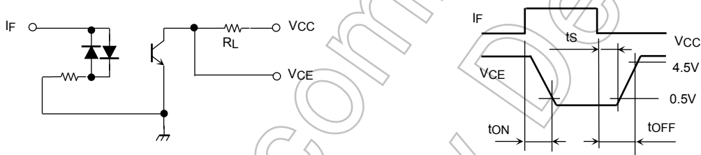
Fig. 1: Switching operating conditions
