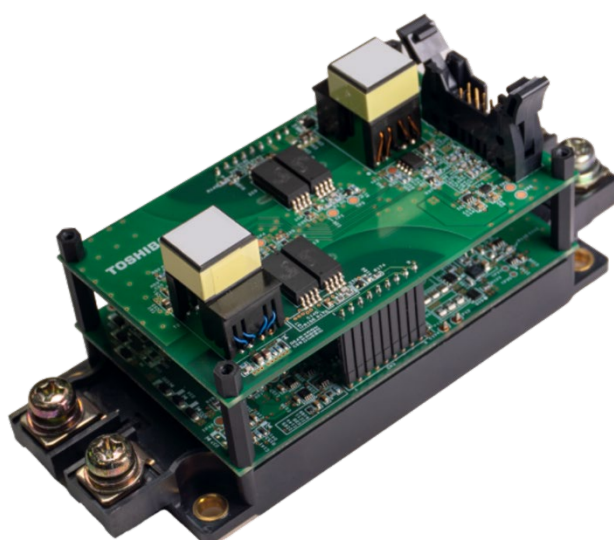
Figure 1.1 This Design Mounted Directly on a Toshiba E3D SiC MOSFET Module
