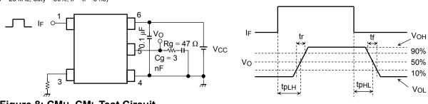
Figure 8: CMH, CML Test Circuit
