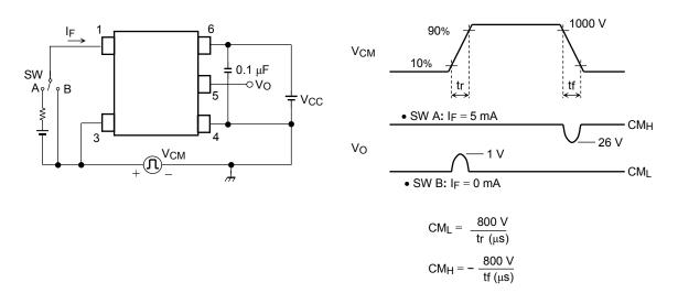
CML (CMH) is the maximum rate of rise (fall) of the common mode voltage that can be sustained with the output voltage in the LOW (HIGH) state.
