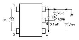
Figure 2: IOPL Test Circuit
