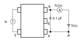
Figure 4: VoL Test Circuit
