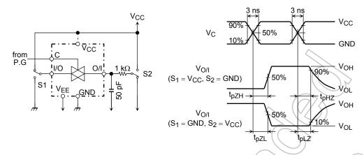
Figure 1  $t_{pLZ}$ ,  $t_{pHZ}$ ,  $t_{pZL}$ ,  $t_{pZH}$
