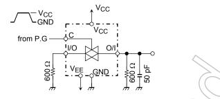
Figure 5 Cross Talk (control input to output signal)
