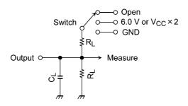
Table 11.7.1 Parameter for AC Test Circuit
