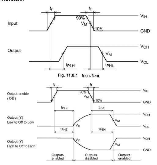
Fig. 11.8.2 t<sub>PLZ</sub>, t<sub>PHZ</sub>, t<sub>PZL</sub>, t<sub>PZH</sub>
