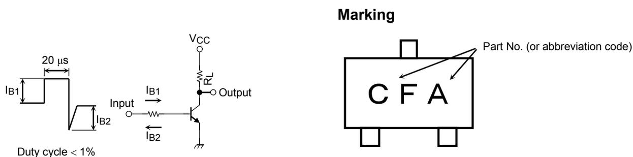
**Figure 1: Switching Time Test Circuit & Timing Chart**
