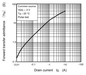
Fig. 7.8 |Y<sub>fs</sub>| - I<sub>D</sub>
