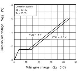
Fig. 7.12 Dynamic Input Characteristics
