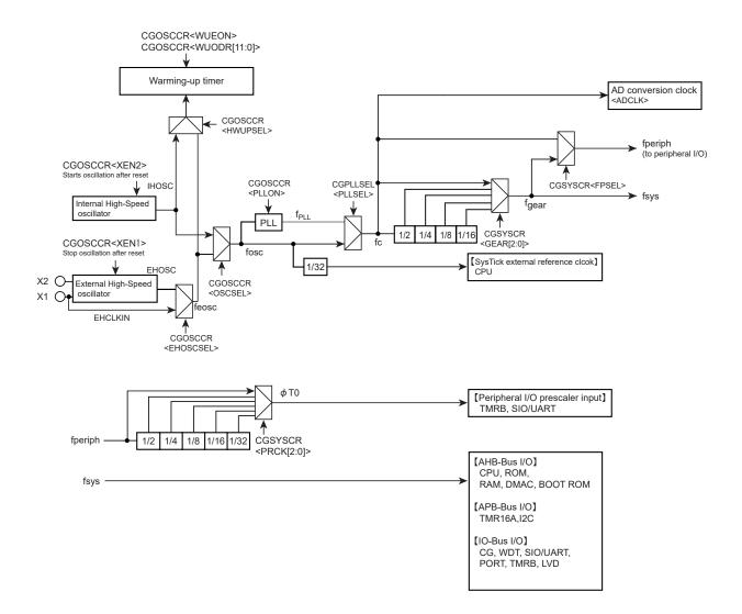
Figure 6-1 Clock Block Diagram
