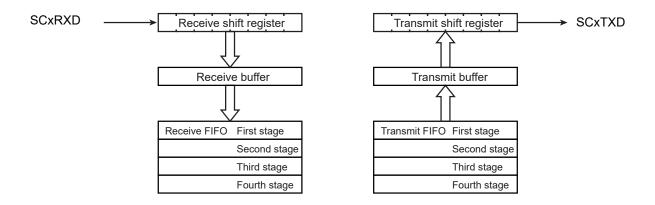
Figure 12-4 The Configuration of Buffer and FIFO
