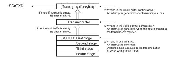
Figure 12-14 Transmit Buffer / FIFO Configuration Diagram
