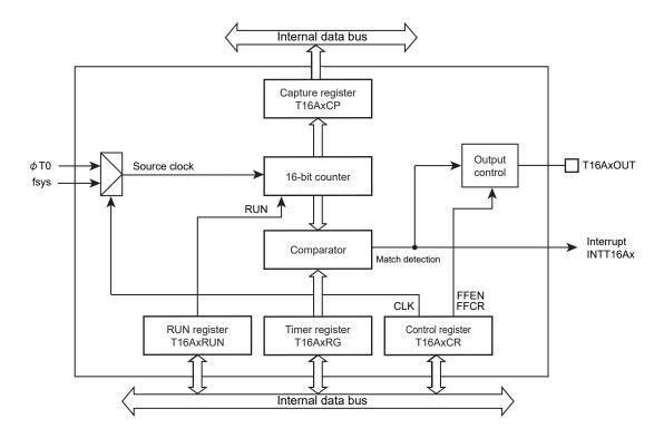
Figure 11-1 Block diagram of TMR16A
