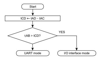
Figure 17-8 Serial operation mode determination flowchart
