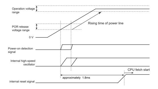
Figure 5-2 Cold reset with power-on-circuit
