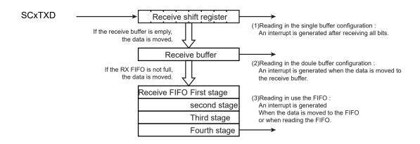
Figure 12-13 Receive Buffer/FIFO Configuration Diagram
