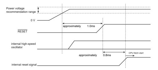
Figure 5-1 Cold reset Operation Sequence
