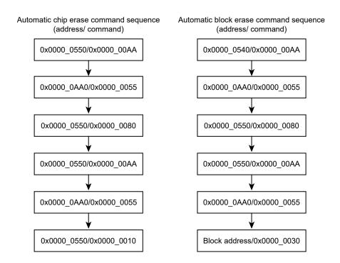
Figure 17-5 Flowchart of automatic erase
