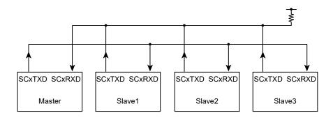
Figure 12-21 Serial Links to Use Wake-up Function
