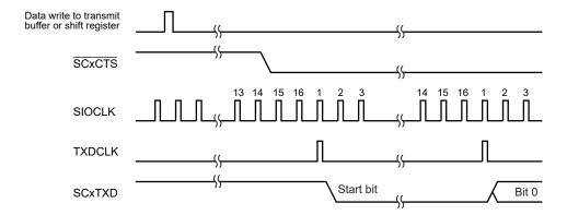
Figure 12-12 SCxCTS Signal timing
