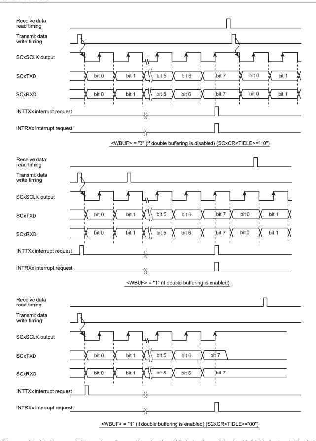
Figure 12-19 Transmit/Receive Operation in the I/O Interface Mode (SCLK Output Mode)
