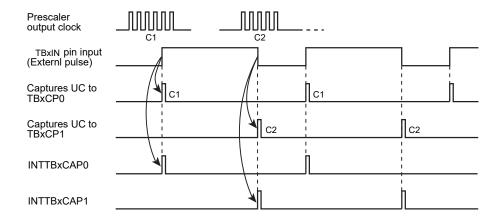
Figure 10-7 Pulse width measurement
