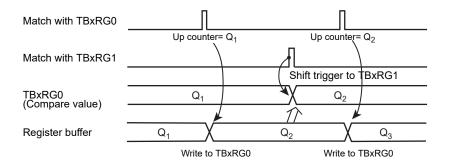
Figure 10-3 Register buffer operation
