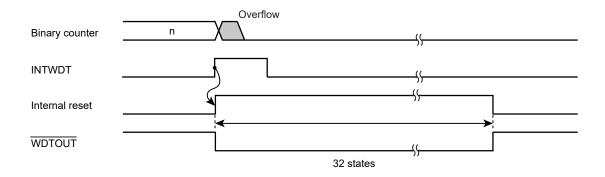
Figure 16-3 Internal reset generation
