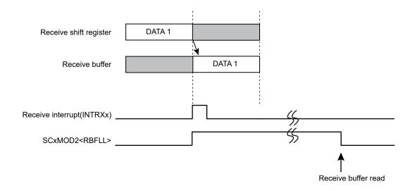
Figure 12-5 Receive Buffer Operation
