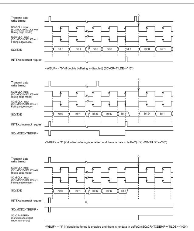
Figure 12-16 Transmit Operation in the I/O Interface Mode (Clock Input Mode)
