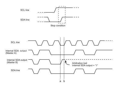
Figure 13-7 Generating the Stop Condition
