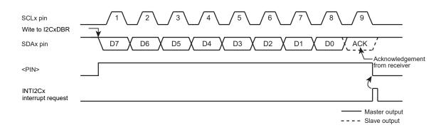
Figure 13-11 <BC[2:0]>= "000", <ACK>= "1" (Transmitter Mode)
