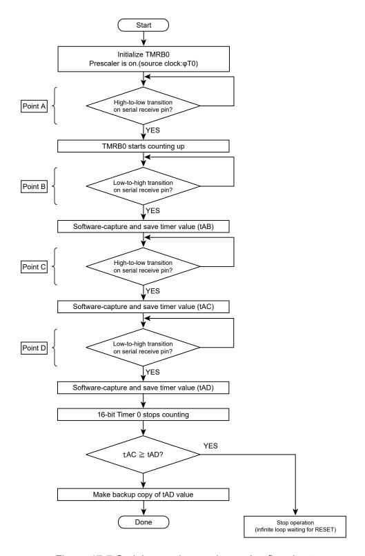
Figure 17-7 Serial operation mode receive flowchart
