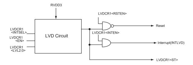
Figure 15-1 LVD Block Diagram
