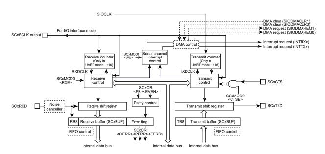
Figure 12-1 Serial Channel Block Diagram
