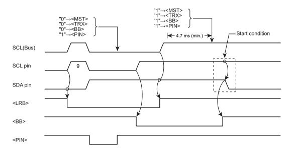
Figure 13-15 Timing Chart of Generating a Restart
