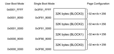
Figure 17-1 Block configuration
