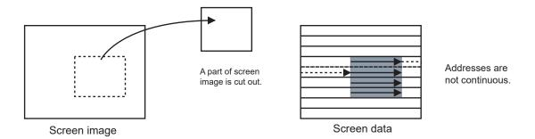
The scatter/gather function can consecutively operate DMA settings (transfer source address, destination address, number of transfers, and transfer bus width) by re-loading them each time a specified number of DMA executions have completed via a pre-set "Linked List" where the CPU does not need to control the operation.
