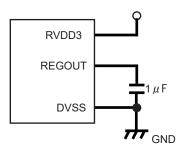
Figure 1-3 Capacitor for a regulator connection circuit
