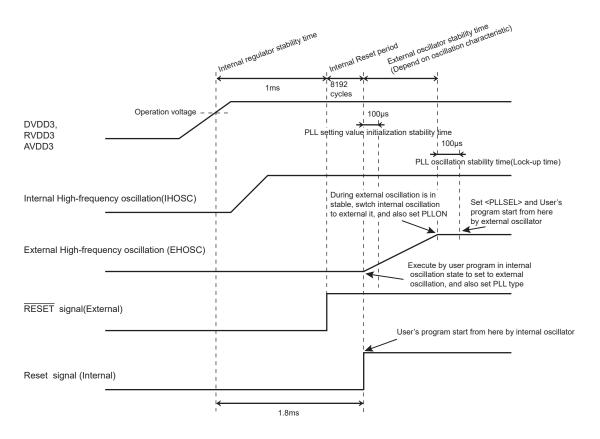
Figure 6-2 Transition when high-speed oscillator is set with PLL
