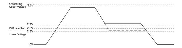
Figure 20-3 Operating Voltage on Startup
