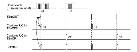
Figure 10-6 Frequency measurement
