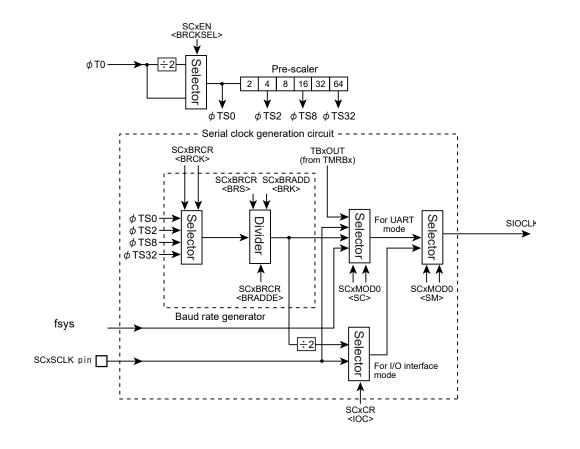
Figure 12-2 Serial clock generation circuit block diagram
