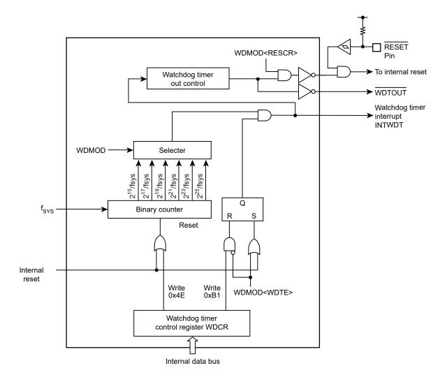
Figure 16-1 Block Diagram of the watchdog Timer
