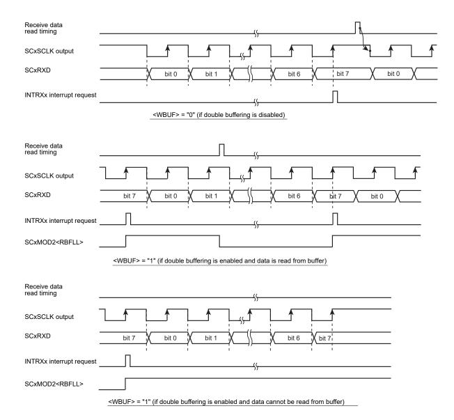
Figure 12-17 Receive Operation in the I/O Interface Mode (Clock Output Mode)
