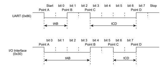
Figure 17-6 Serial operation mode determination data
