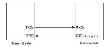
Figure 12-11 Handshake Function
