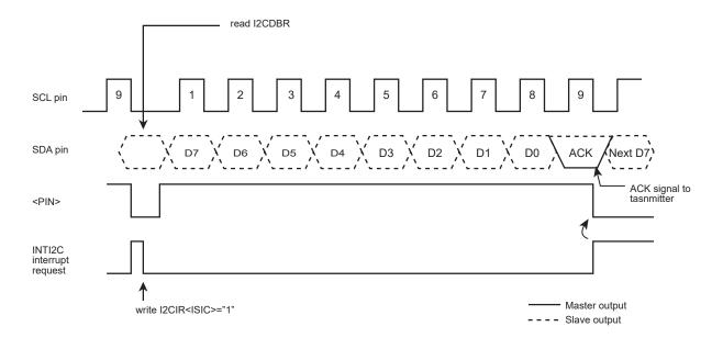
Figure 13-12 <BC[2:0]>= "000",<ACK>= "1" (Receiver Mode)
