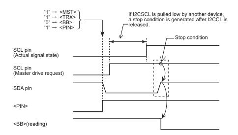
Figure 13-14 Generating the Stop Condition
