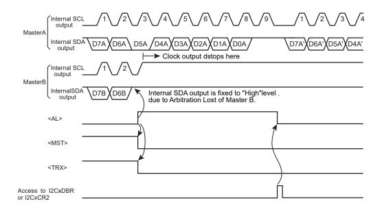
Figure 13-9 Example of Master B Lost Arbitration (D7A = D7B, D6A = D6B)
