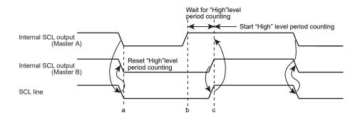
Figure 13-5 Example of Clock Synchronization
