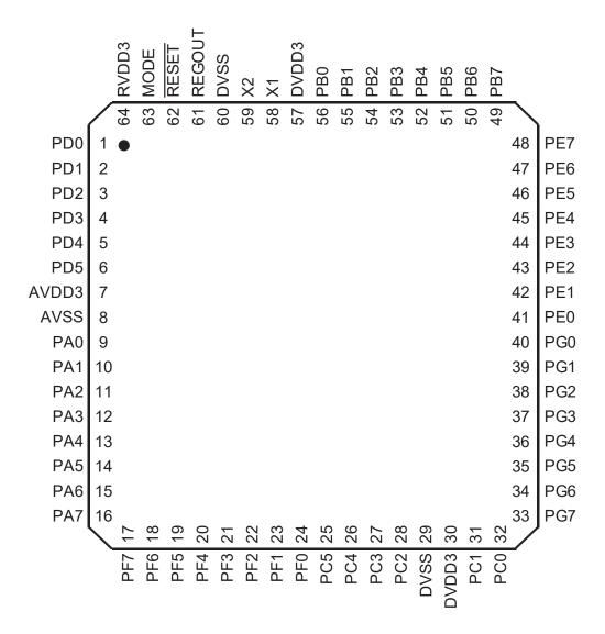
Figure 1-2 Pin Layout (LQFP64 TOP VIEW)
