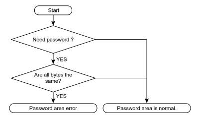
Figure 17-10 Password area check flowchart
