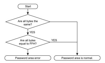
Figure 17-9 Password area check flowchart
