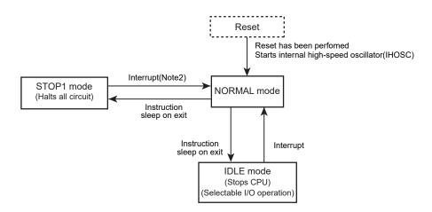
Figure 6-3 Mode Transition Diagram
