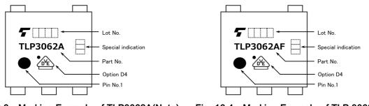
Fig. 16.3 Marking Example of TLP3062A(Note)
