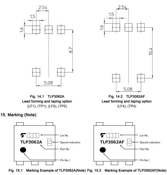
Note: A different marking is used for photocouplers that have been qualified according to option (D4) of EN 60747. See Fig.16.3 and Fig.16.4.
