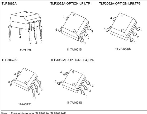
Note: Through-hole type: TLP3062A, TLP3062AF Lead forming option: (LF1), (LF4), (LF5) Taping option: (TP1), (TP4), (TP5)
