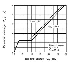
Fig. 8.9 Dynamic Input Characteristics
