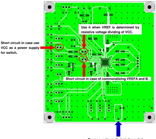
Power supply applied pin for switch (Apply 3.3 V or 5 V in necessary.)
