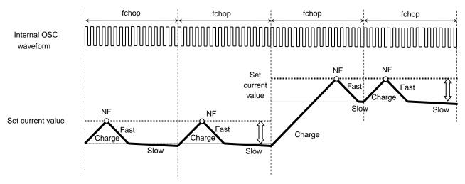
Figure 5.3 ADMD current waveform
