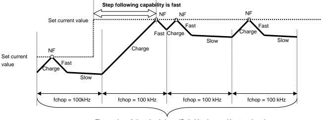
The number of chopping is large (Switching loss and heat are large)
