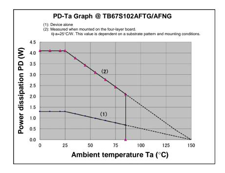
Figure 10.1 Power dissipation
