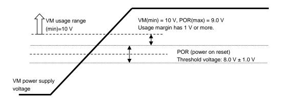
Figure 1.1 Power supply voltage and usage range
