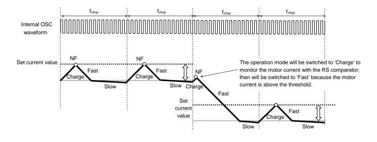
Figure 5.5 ADMD current waveform (When the next current step is lower)
