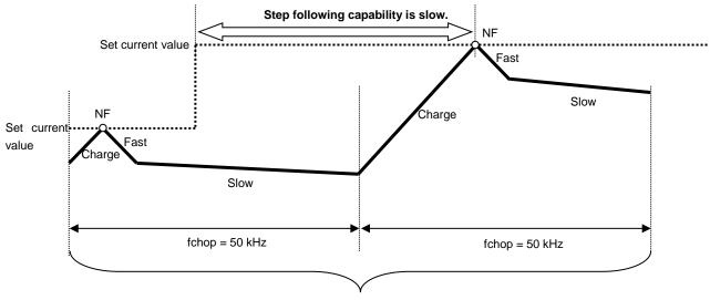
The number of chopping is small (Switching loss and heat are small)
