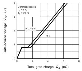
Fig. 9.1.9 Dynamic Input Characteristics
