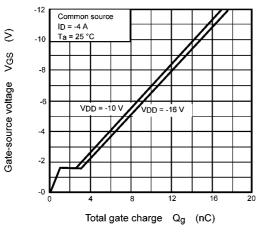
Fig. 9.2.9 Dynamic Input Characteristics
