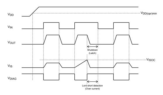
Note: Output shut down when it detects short circuit and becomes latch state and protects outside MOSFET.
