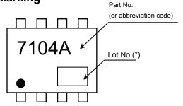
Note: • on the lower left of the marking indicates Pin 1
