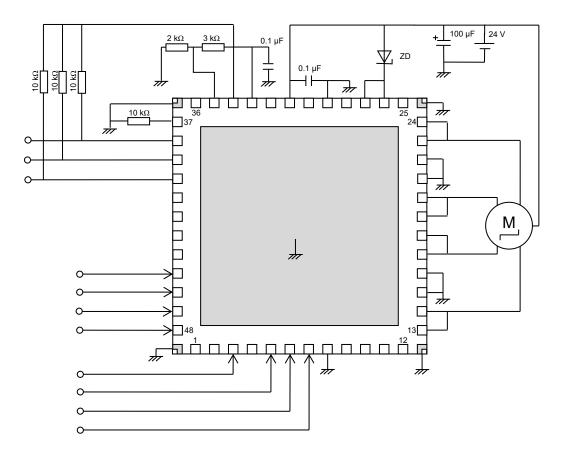
Figure 10.1 Application Circuit Example (Constant current control)
