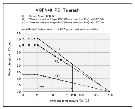
Figure7 (For reference) PD-Ta graph
