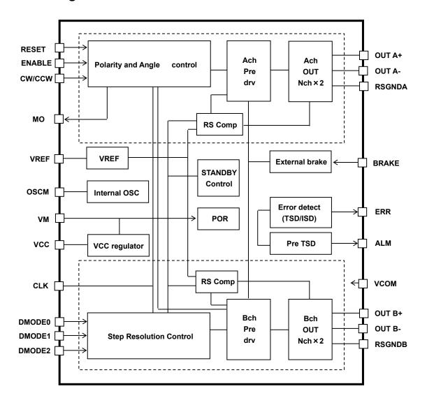
Figure 3.1 Block Diagram
