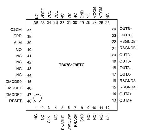
Figure 4.1 Pin Assignments (top view)
