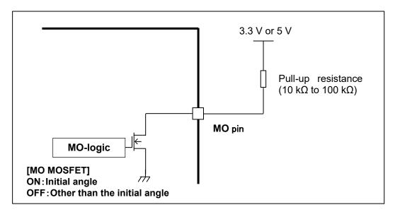
Figure 6.2 Monitor pin equivalent circuit
