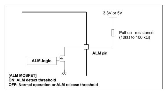
Figure 6.5 ALM pin equivalent circuit
