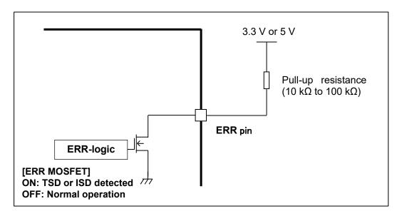
Figure 6.3 ERR pin equivalent circuit
