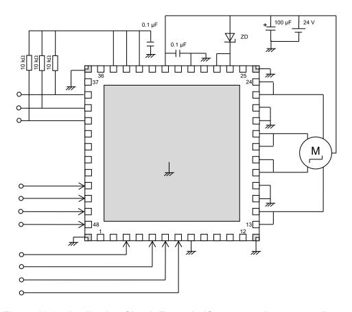
Figure 10.2 Application Circuit Example (Constant voltage control)
