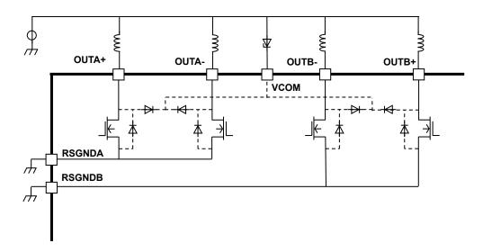
Figure 6.1 BRAKE mode equivalent circuit
