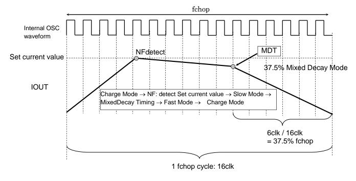
Figure 5.1 Current waveform of Mixed Decay Mode
