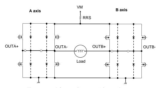
Figure 7.2 1 DC motor (Large mode) operation
