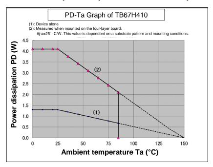
Figure 10.1 Power dissipation
