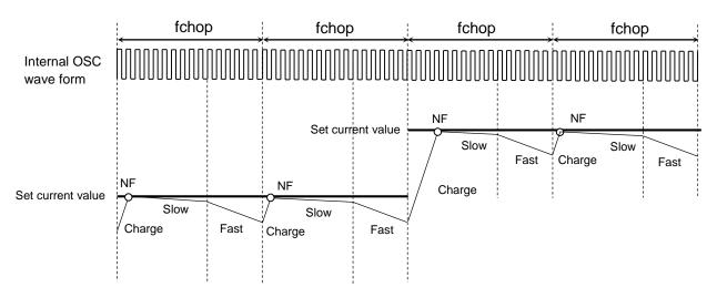
Figure 5.2 Current waveform in Mixed Decay Mode (When current value increases)
