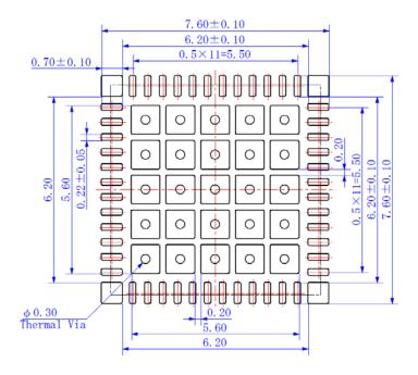
Figure 11.1 QFN48 foot pattern
