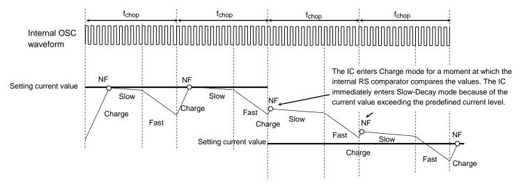
Figure 5.3 Current waveform in Mixed Decay Mode (When a current value decreases)
