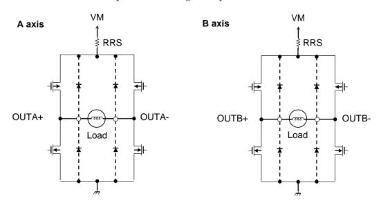
Figure 7.1 2 DC motors (Small mode) operation
