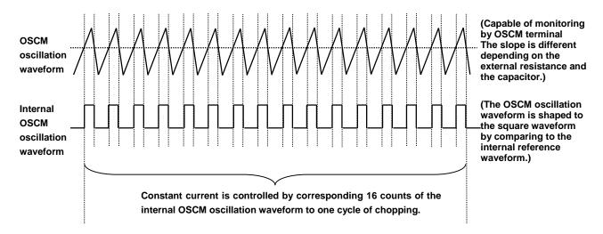
Figure 4.1 OSCM oscillation frequency
