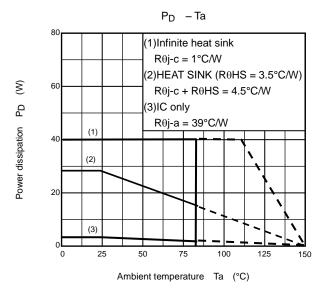
PD-Ta curve of the TB67H302HG in each mounted condition are shown below.
