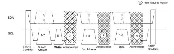
Figure 7-1 Bus control timing (Basic mode)
