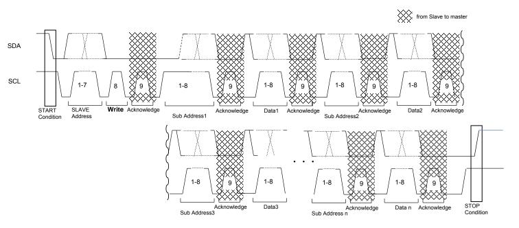
Figure 7-2 Bus control timing (Write mode)
