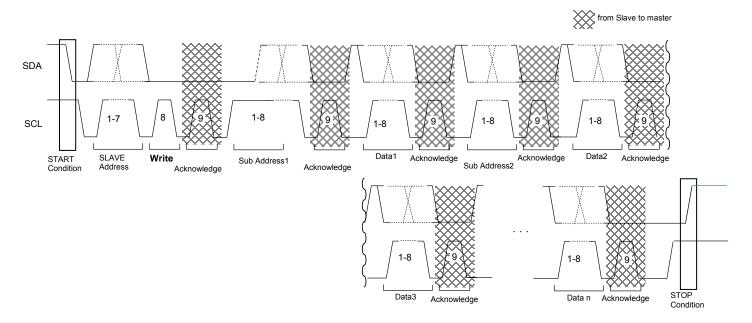
Figure 7-3 Bus control timing (auto increment mode)
