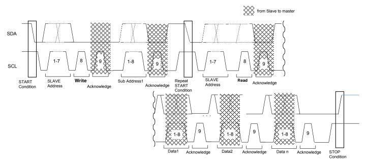
Figure 7-4 Bus control timing (Read mode)
