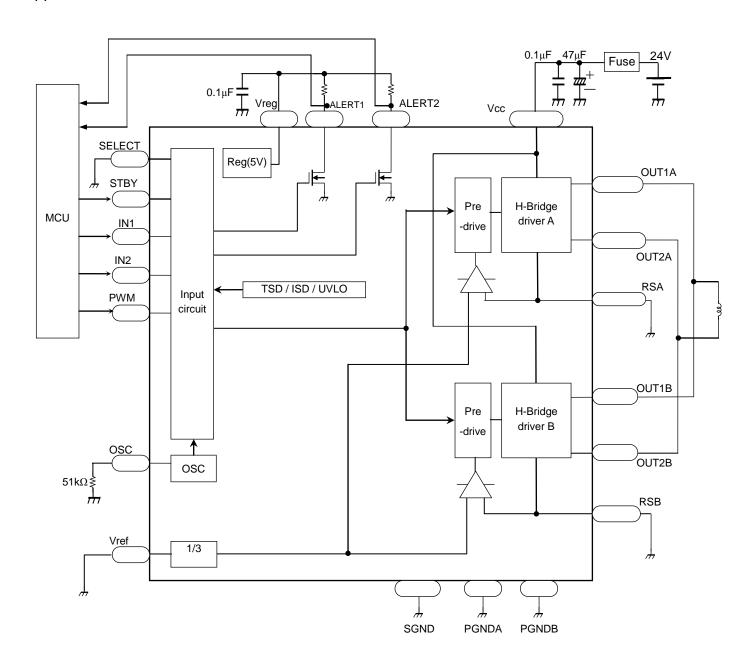
Set SELECT "L" in direct PWM drive. RSA should be connected to PGNDA. RSB should be connected to PGNDB. Vref should be connected to SGND.
