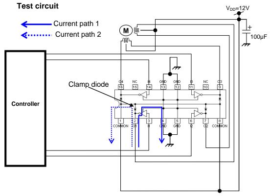
When clamp diode and zener diode are used.
