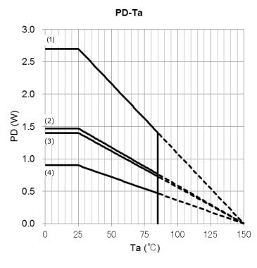
(1)When mounted on DIP16 type (50×50×1.6mm Cu 50%, single-side glass epoxy) (2)DIP16 type alone (3)When mounted on HSOP16 / SSOP24 (60×30×1.6mm Cu 30%, single-side glass epoxy) (4)HSOP16/SSOP24 type alone
