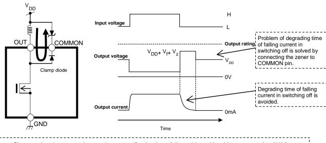
Please select the zener whose voltage specification is as follows;  $V_{DD} + V_Z + V_f <$  output rating (50V)
