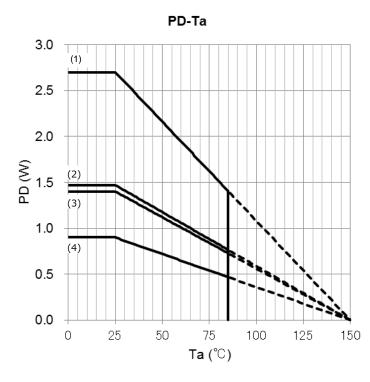
(1)When mounted on DIP16 type (50x50x1.6mm Cu 50%, single-side glass epoxy) (2)DIP16 type alone (3)When mounted on HSOP16 / SSOP24 (60x30x1.6mm Cu 30%, single-side glass epoxy) (4)HSOP16/SSOP24 type alone
