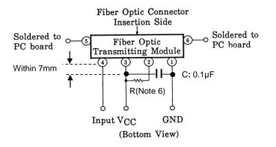
Note 6: Select a resistor value as follows: (with TORX1951A(F))
