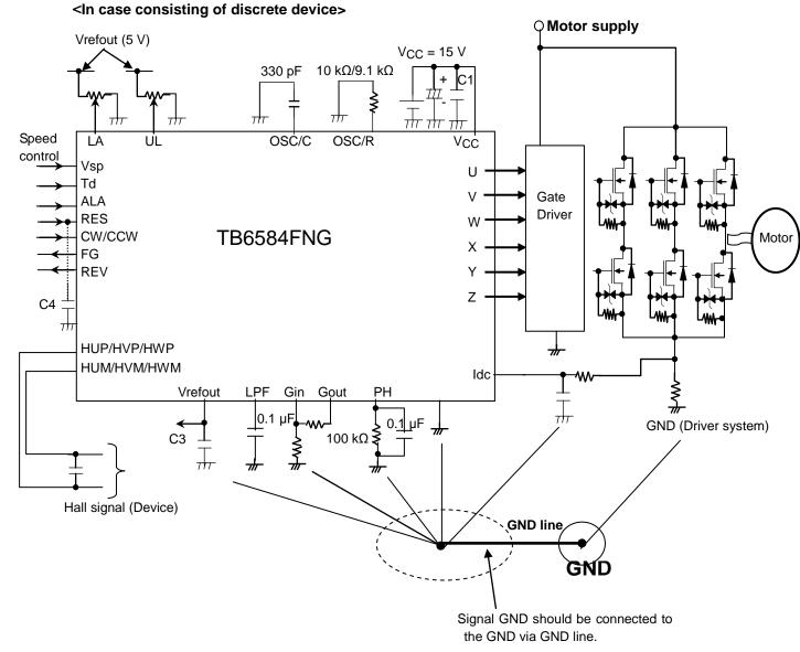
Note) The operation of TB6584FNG is controlled by synchronous rectification in sine-wave driving mode. OFF time of upper phase (U, V, and W) and lower phase (X, Y, and Z) is controlled about 2 µsec. So, please make sure to control the switch speed of the gate driver and the discrete device. When the response speed is low, there is a possibility that the device is destroyed by rush current which is generated by turning on the upper and lower phase at the same time.
