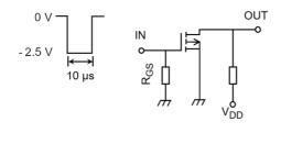
Fig. 5.3.1 Switching Time Test Circuit
