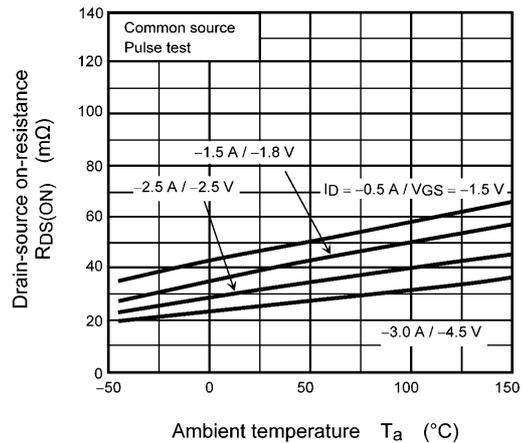
**Fig. 8.6**  $R_{DS(ON)} - T_a$
