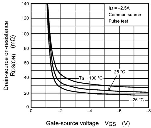
**Fig. 8.4**  $R_{DS(ON)} - V_{GS}$
