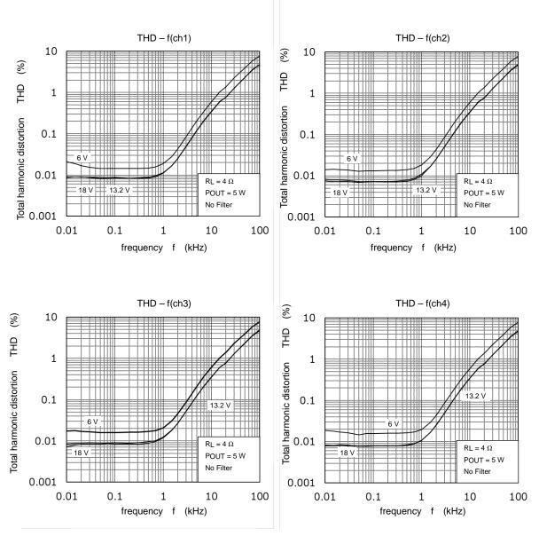
Figure 13-3 Frequency Characteristics of Total Harmonic Distortion
