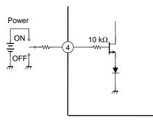
Figure 1 Internal circuit for standby
