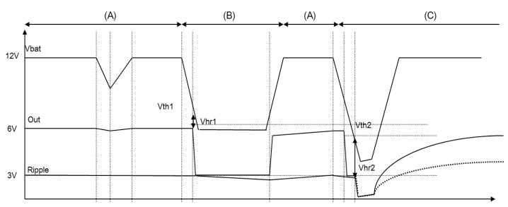
Figure 12 Output VDD/2 voltage in lowering VDD
