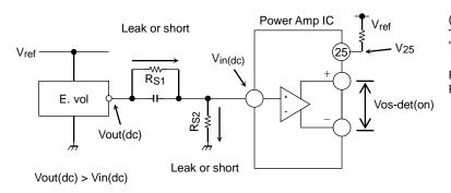
(Reference) The specification defines the Offset voltage as "OUT(+) - OUT(-)"
