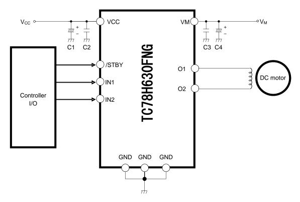
All the grounding wires of the device must run on the solder mask on the PCB and be externally terminated at only one point.
