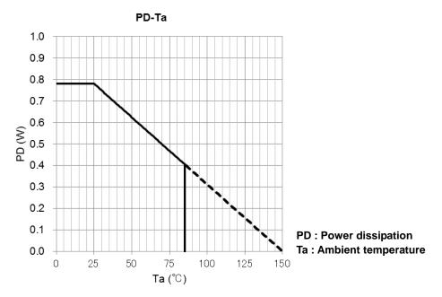
When mounted on a glass epoxy board (50 mm × 50 mm × 1.6 mm, Cu area: 40 %, Cu thick: 35 µm)
