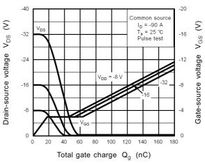
Fig. 8.14 Dynamic Input/Output Characteristics
