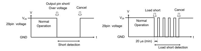
Figure 7.10 Pin 29 output waveform
