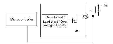
Figure 7.9 Generating mechanism of output short detection
