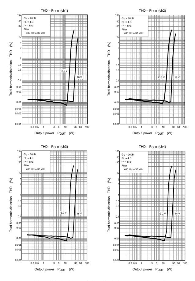
Figure 13.2 Total Harmonic Distortion by Power-supply Voltage ( $R_L = 4 \Omega$ )
