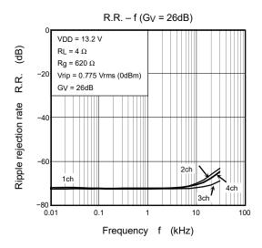
Figure 13.5 Frequency Characteristics of Ripple Rejection Rate
