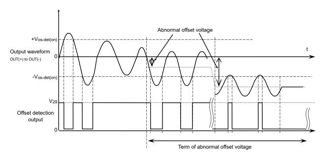
Figure 7.8 Output waveform of Pin 29
