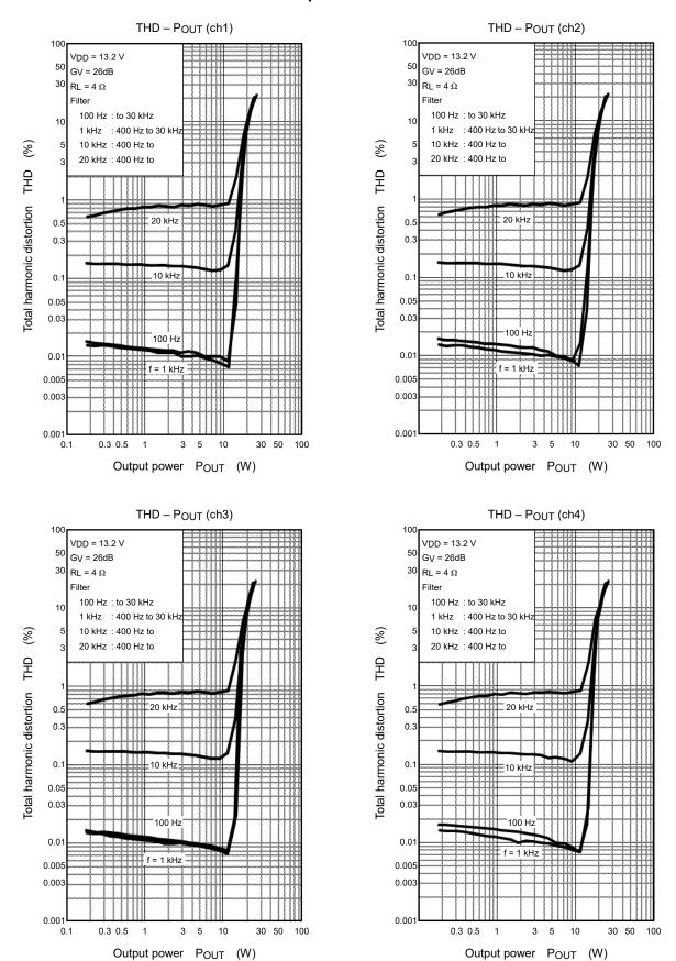
Figure 13.1 Total Harmonic Distortion of Each Frequency ( $R_L = 4 \Omega$ )
