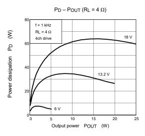
Figure 13.8 Power Dissipation vs. Output Power
