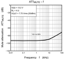
Figure 13.4 Frequency Characteristics of Voltage Gain and Mute Attenuation
