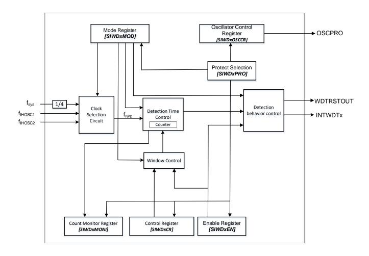
Figure 2.1 SIWDT block diagram
