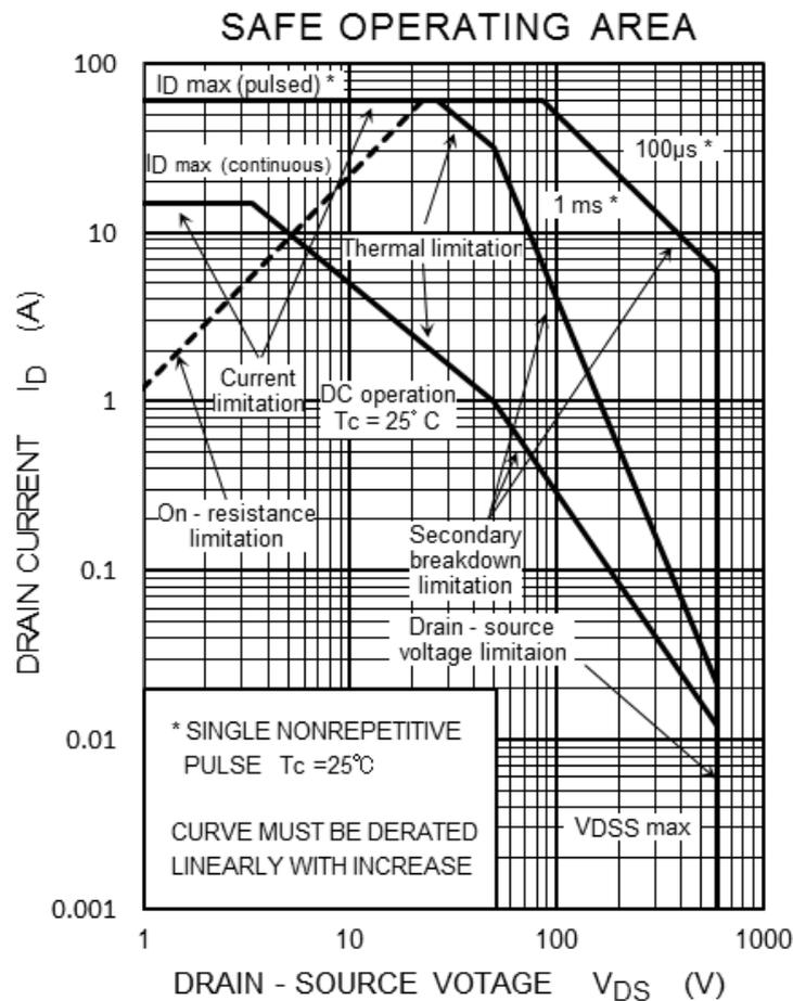
Figure 2.1 Safe operating area of a MOSFET
