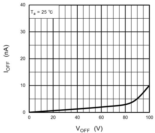
Fig. 16.1.10  $I_{OFF} - V_{OFF}$
