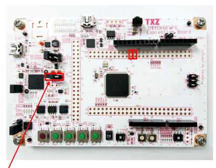
CN18: External power should be supplied to No2 pin.
