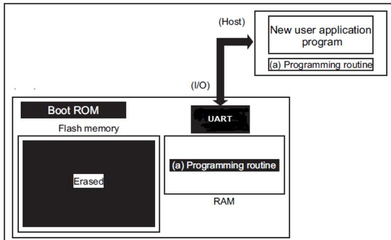
**Figure 6.22 Procedure of Using Reprogramming Algorithm in Boot ROM (4)**
