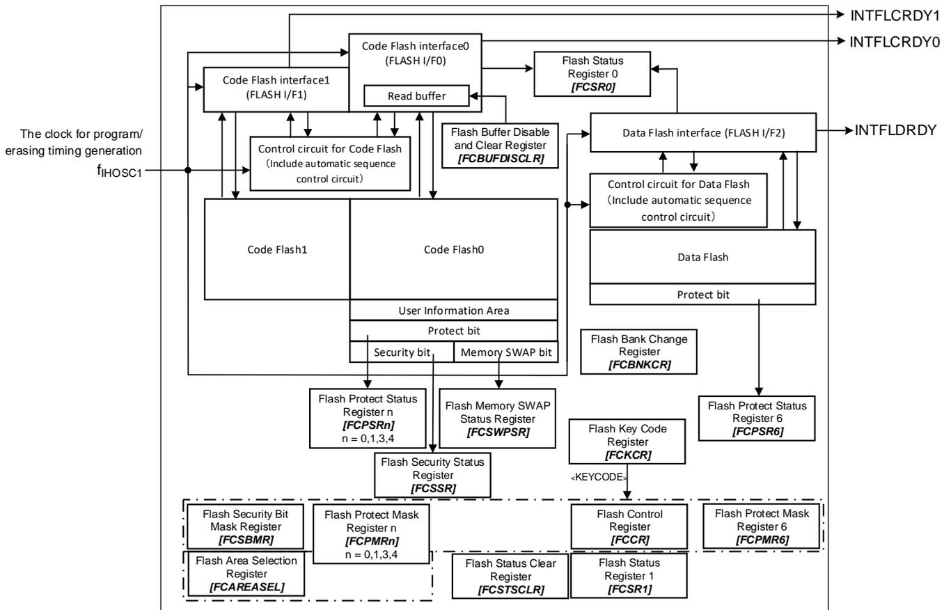
**Figure 2.1 The Block Diagrams of a flash memory**
