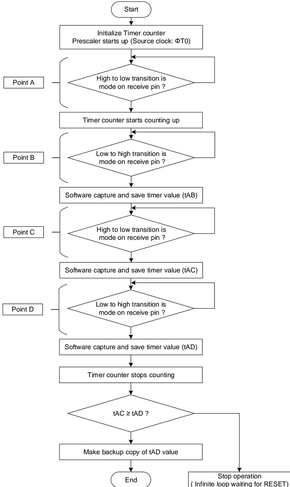
Figure 6.14 Reception flowchart in serial operation mode
