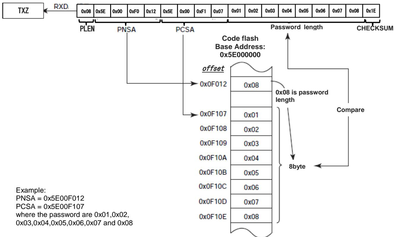
Figure 6.16 Password configuration (Example of Transmission)
