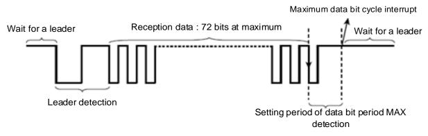
Figure 3.1 Data reception completes by detecting the maximum data bit cycle
