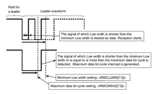
Figure 3.9 Leader-less remote control signal during the leader wait state (In the case of [RMCxRCR2]<RMCLD> = 1)
