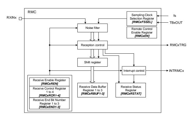
The block diagram of RMC is shown in the following figure.
