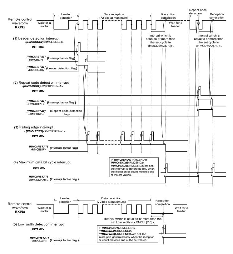
Figure 3.8 shows the waveform of the remote control signals and the interrupt generation timings.
