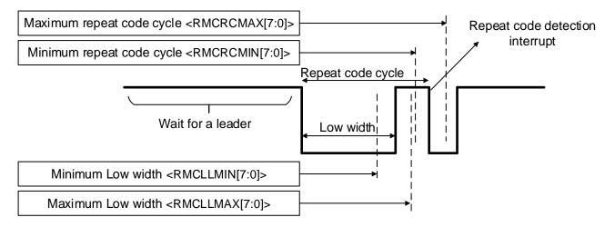
Figure 3.4 Repeat code waveform and registers [RMCxRCR1] and [RMCxRCR3]
