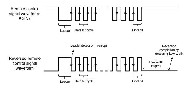
Figure 3.10 Reception of the remote control signal which starts with Low width only leader
