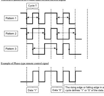
Waveform patterns of Phase-type remote control signal
