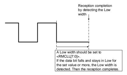
Figure 3.7 Reception completion by detecting Low width
