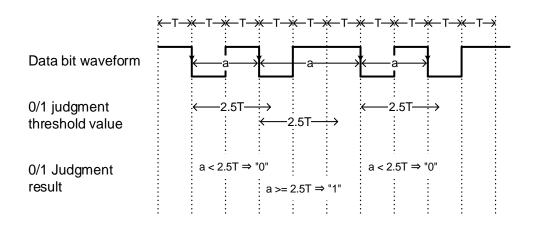
Figure 3.5 0/1 judgment of a data bit (Threshold value: 2.5T)
