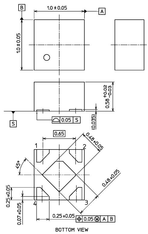
0.04 mm (typ.) unevenness exists along the edges of the back electrode to increase shear after soldering.
