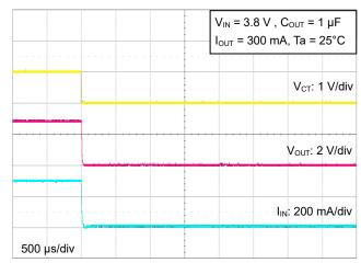
Note: The above characteristics curves are presented for reference only and not guaranteed by production test, unless otherwise noted.
