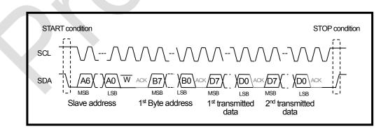
Figure 4-16 I<sup>2</sup>C transfer format (write 2-byte data to serial memory write)
