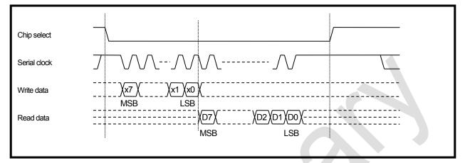
Figure 4-11 SPI format (Single Byte read)
