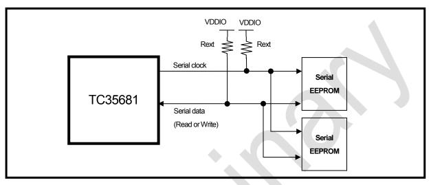
Figure 4-13 Example of the connection with serial EEPROM's through I<sup>2</sup>C interface (open-drain output mode)
