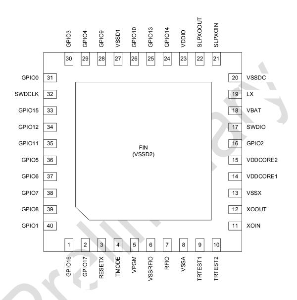
Figure 2-1 Pin assignment of TC35681IFTG (Top view)
