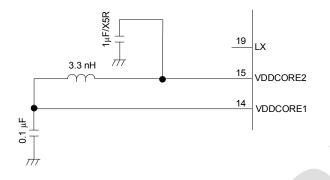
Figure 6-3 Circuit for LDO regulator
