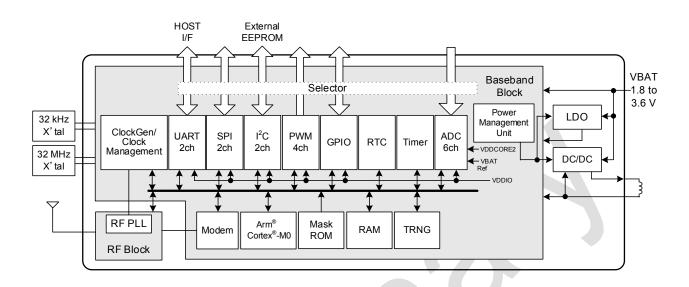
Figure 3-1 Internal block diagram of TC35681 and an example of connection of main components
