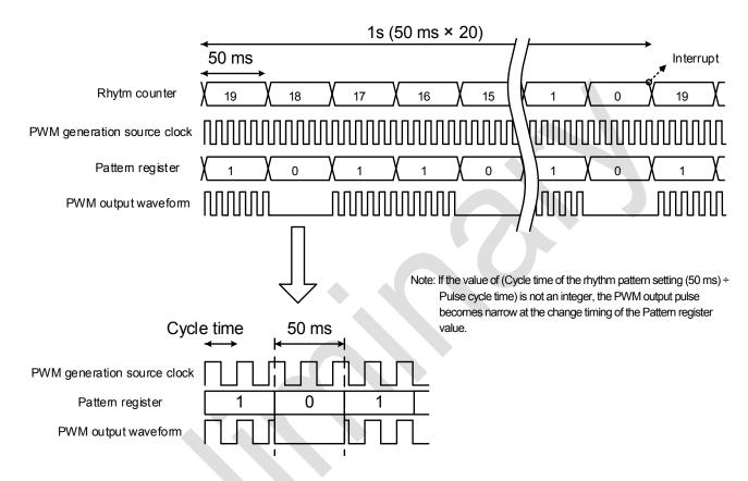
Figure 4-18 Output masking by PWM rhythm function
