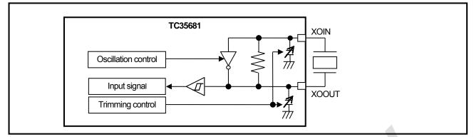
Figure 4-20 Connection of a crystal resonator
