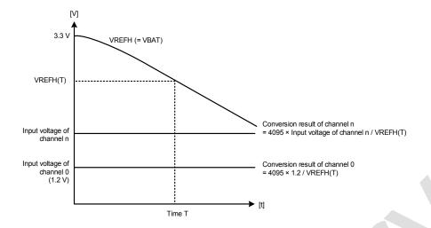
Figure 4-19 Conceptual diagram of the voltage conversion
