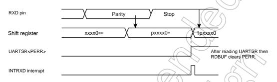
Figure 11-5 Generation of Parity Error
