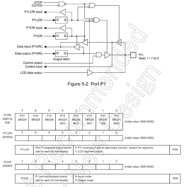
Note: The port placed in input mode reads the pin input state. Therefore, when the input and output modes are used together, the output latch contents for the port in input mode might be changed by executing a bit manipulation instruction.
