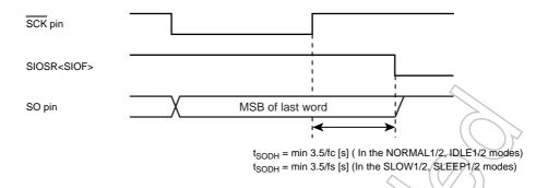
Figure 12-9 Transmiiied Data Hold Time at End of Transfer
