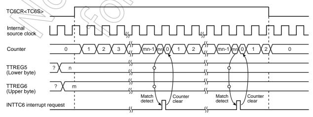
Figure 10-6 16-Bit Timer Mode Timing Chart (TC5 and TC6)
