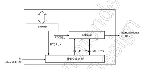
Figure 16-1 Configuration of the RTC
