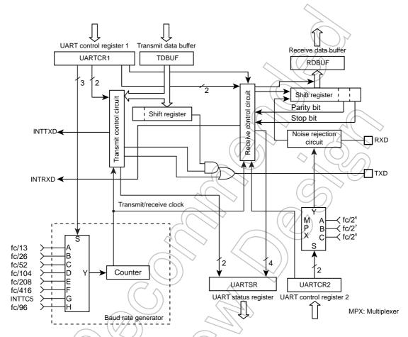
Figure 11-1 UART (Asynchronous Serial Interface)
