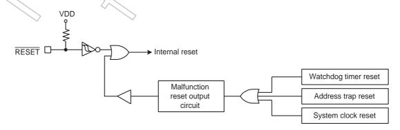
Figure 2-15 Reset Circuit
