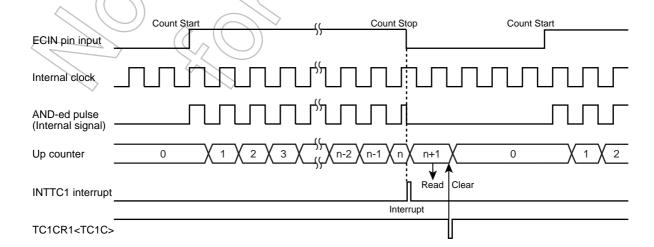
Figure 8-4 Pulse width measurement mode timing chart
