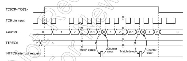
Figure 10-3 8-Bit Event Counter Mode Timing Chart (TC6)
