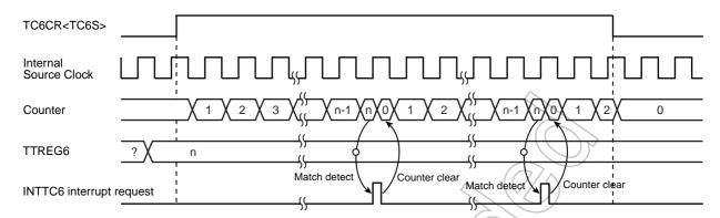
Figure 10-2 8-Bit Timer Mode Timing Chart (TC6)
