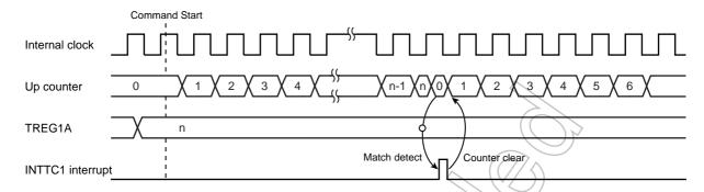
Figure 8-2 Timing chart for timer mode
