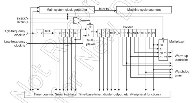
Figure 2-4 Configuration of Timing Generator
