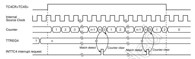
Figure 9-2 8-Bit Timer Mode Timing Chart (TC4)
