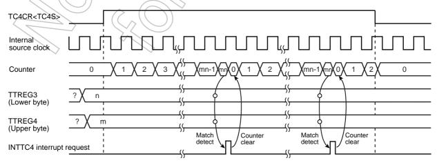
Figure 9-6 16-Bit Timer Mode Timing Chart (TC3 and TC4)
