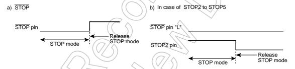
Figure 14-3 Priority of STOP pin and STOP2 to STOP5 pins
