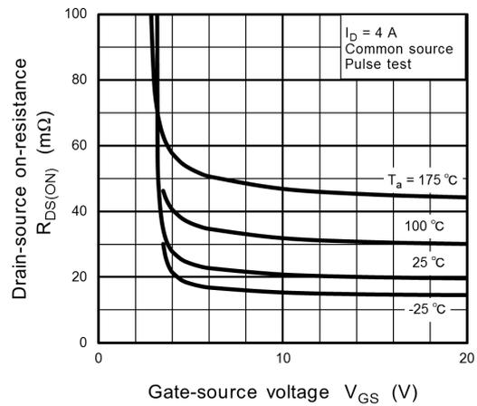
**Fig. 9.4  $R_{DS(ON)} - V_{GS}$**
