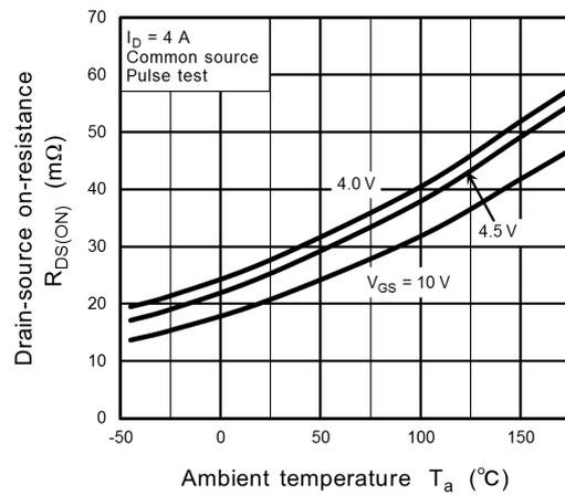
**Fig. 9.6  $R_{DS(ON)} - T_a$**
