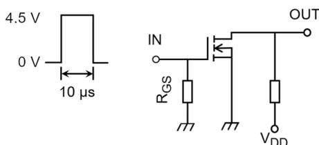
Fig. 7.3.1 Switching Time Test Circuit
