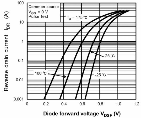
**Fig. 9.8  $I_{DR} - V_{DSF}$**
