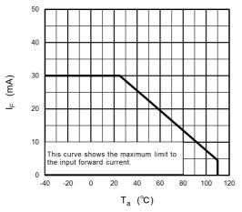
Fig. 12.1.1 I<sub>F</sub> - T<sub>a</sub>
