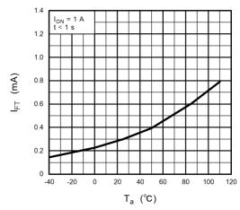
Fig. 12.1.6 I<sub>FT</sub> - T<sub>a</sub>
