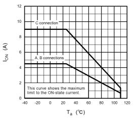
Fig. 12.1.2 I<sub>ON</sub> - T<sub>a</sub>
