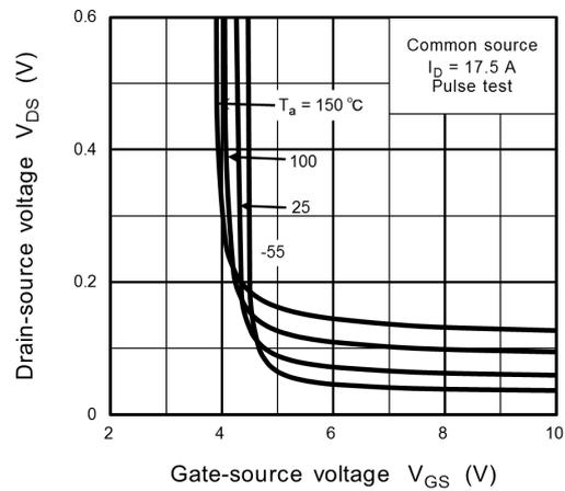
**Fig. 8.4  $V_{DS} - V_{GS}$**
