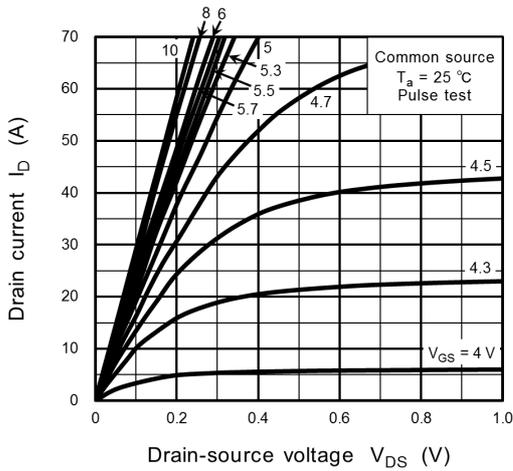
**Fig. 8.1  $I_D - V_{DS}$**
