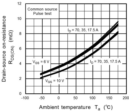
**Fig. 8.9  $R_{DS(ON)} - T_a$**
