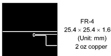
Fig. 5.1 Device Mounted on a Glass-Epoxy Board (a)
