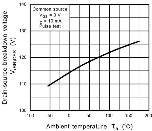
**Fig. 8.11  $V_{(BR)DSS} - T_a$**
