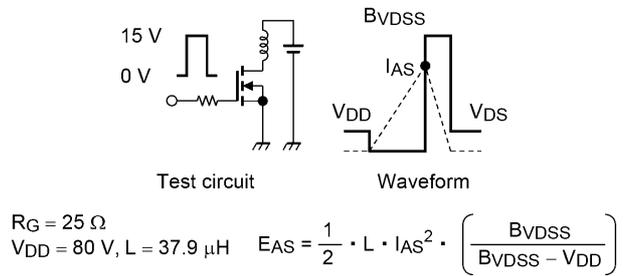
**Fig. 8.16 Test Circuit/Waveform**
