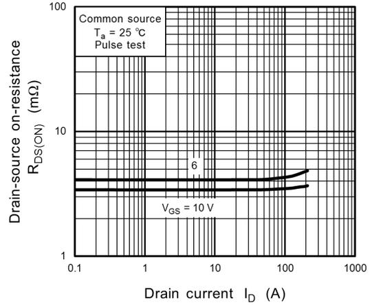
**Fig. 8.8  $R_{DS(ON)} - I_D$**
