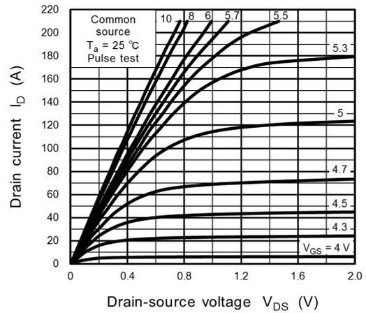
**Fig. 8.2  $I_D - V_{DS}$**
